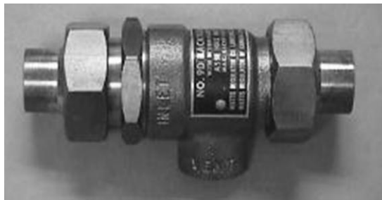
ASSE 1012 Dual Check with Vent Low hazard only – not on hose bibs
