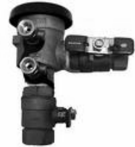
ASSE 1020 Pressure Vacuum Breaker Only for backsiphonage; used for sprinkler systems with shut offs downstream; outside installation
